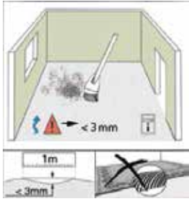
Fig 1. Ensure that the subfloor is clean and level. Using a 1 metre straightedge, the subfloor level should not exceed 3mm over 1 metre in any direction. Uneven subfloors will effect the performance of the product and may lead to product failure. Uneven floors can also cause noise. Floors can be levelled with a self leveling compound and high spots can be ground/sanded. The product can be installed over well adhered and level vinyl, cork, ceramic tiles and timber floorcoverings (never over other floating floorcoverings) The product cannot be installed over carpet and or carpet underlay.
